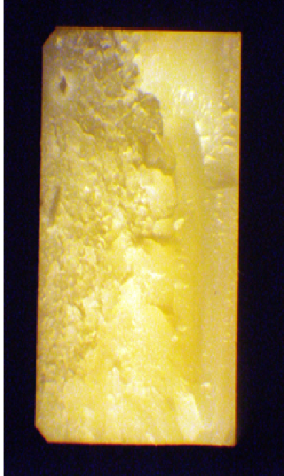
Fractured surface after impact (4x6 mm)
