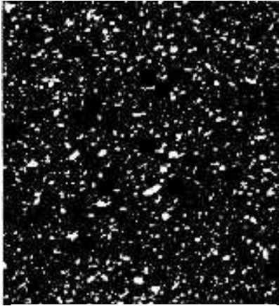
Distribution of additives (white dots) in PVC matrix; surface shown: ca. 0.2x0.2 mm
